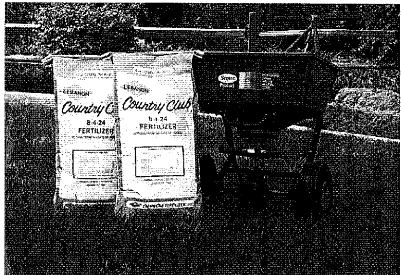
FIGURE 2. A rotary (broadcast) spreader for rapid application of fertilizer to small or medium-sized turf areas.
