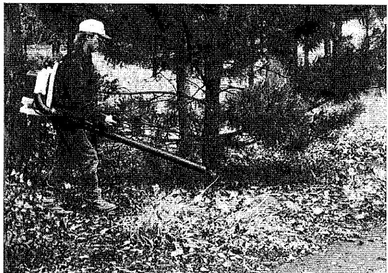
FIGURE 4. A backpack blower uses air speed to move dust, dirt, leaves, and grass clippings.
